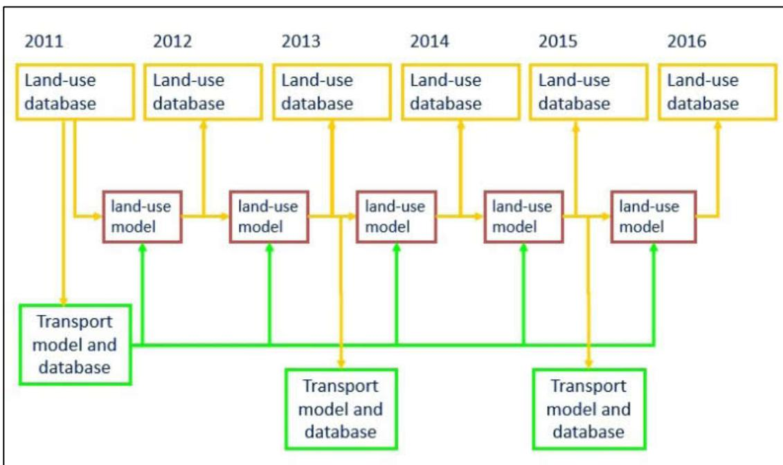
Figure 6 - Time series marching in a TILU model
